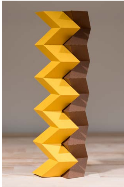
Figure 1: Paper model of the original “zipper” coupled origami tubes. Photo courtesy of Rob Felt.
